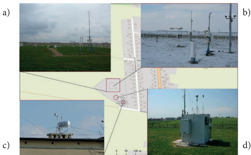
Fig. 5: Location of measuring equipment at the meteorological and aerosol monitoring station in Ratibor Studzienna: (a) meteorological garden; (b) ceilometer; (c) radiometer; (d) aerosol measuring container.
